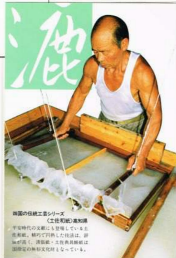
Dipping and lifting the mould Japan postal stationery card
